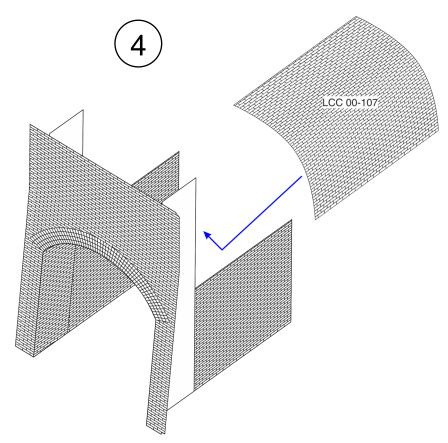
Pre bend LCC 00-107 and insert into the archway. Ensure there is no gaps between the brickwork by gently pushing it in with pointy object (e.g. back of a hobby knife).
